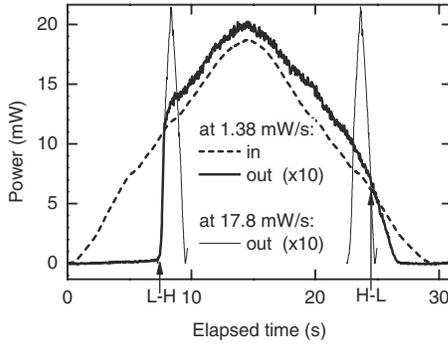
FIG. 3. Temporal profile of the power of incident (dashed line) and transmitted (solid thick line, with  $10\times$  magnification) beams at slow sweeping speed, under exposure to 100% ethanol concentration. The transmitted beam at the highest sweep speed is also shown for comparison (solid thin line, shown twice to facilitate the visual comparison of the rising and falling fronts with the slow sweeping case).
