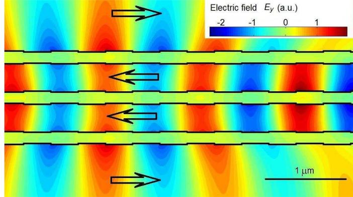
Fig. 5. Snapshot of the electric field  $E_y$  distribution, according to 2D FDTD simulation of the structure in Figure 2, with 100 periods, and with supermode  $+-$  excitation (see Figure 1). Light is injected from the left side. Excitation is narrowband (vacuum wavelength  $\lambda_0 \approx 1.54 \mu\text{m}$ ). Only a few periods are shown, in proximity of the input side. Map is to scale. Large arrows indicate the direction of energy flux (Media 1).
