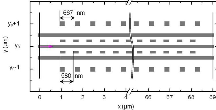
Fig. 6. Sample 2D photonic structure to selectively filter supermode  $+++$  or supermode  $+-$  (supermode profiles are shown in Figure 1). Grey (white) areas represent Si (air). The vertical line at  $x = 0 \mu\text{m}$  indicates the location of the energy source in FDTD simulations. The arrow indicates the direction of injection. The vertical line at  $x = 69 \mu\text{m}$  indicates the location of monitor. The graph is to scale.
