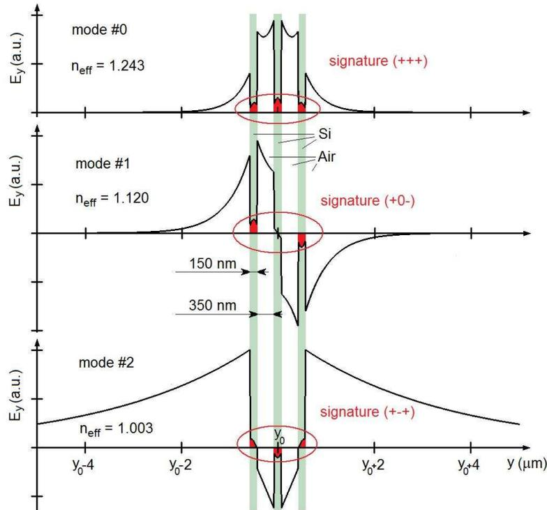
Fig. 1. Signatures of the 3 guided TM supermodes at vacuum wavelength  $\lambda_0=1.55 \mu\text{m}$  in a 2-slot waveguide resulting from 3 coupled 150 nm thick Si slabs. Air slots are 350 nm thick. For each supermode, the effective index  $n_{\text{eff}}$  is also shown. The thickness of Si slabs is chosen to guarantee single mode operation (for the isolated slab).
